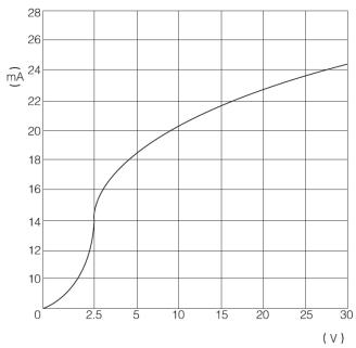
Input Current v. Control Voltage: 90 ~ 250VAC
