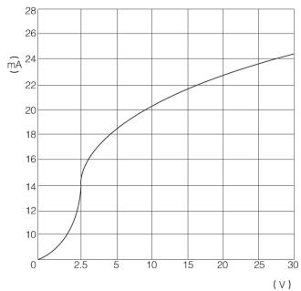
Input Current v. Control Voltage: 90 ~ 250VAC
